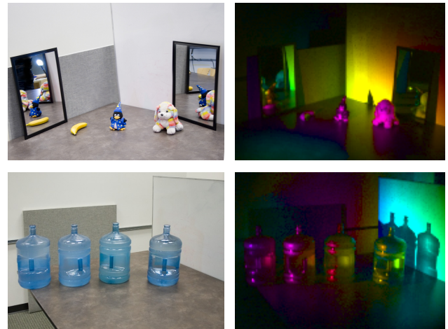
Figure 11: Our test scenes. All scenes are illuminated from the left, with the rainbow images encoding the temporal location of the main intensity peak for each pixel. Top: Various objects on a table, and their reflections in mirrors placed nearby. Note how the items and mirrored counterparts light up at different times. Bottom: Four bottles filled with slightly scattering water. The specular reflections reach the camera before the light scattered inside the bottles.
